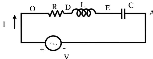
**Fig. 15.1 (a) Circuit diagram**
